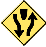
Divided Highway (Road) Begins
